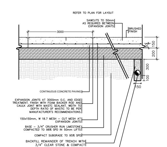
NOTE: -ALL DIMENSIONS ARE IN MILLIMETERS - PROVIDE EXPANSION JOINTS AS PER SITE DIRECTION BY LANDSCAPE ARCHITECT - PLACE DRAINS AS PER SITE SERVICING DRAWINGS
