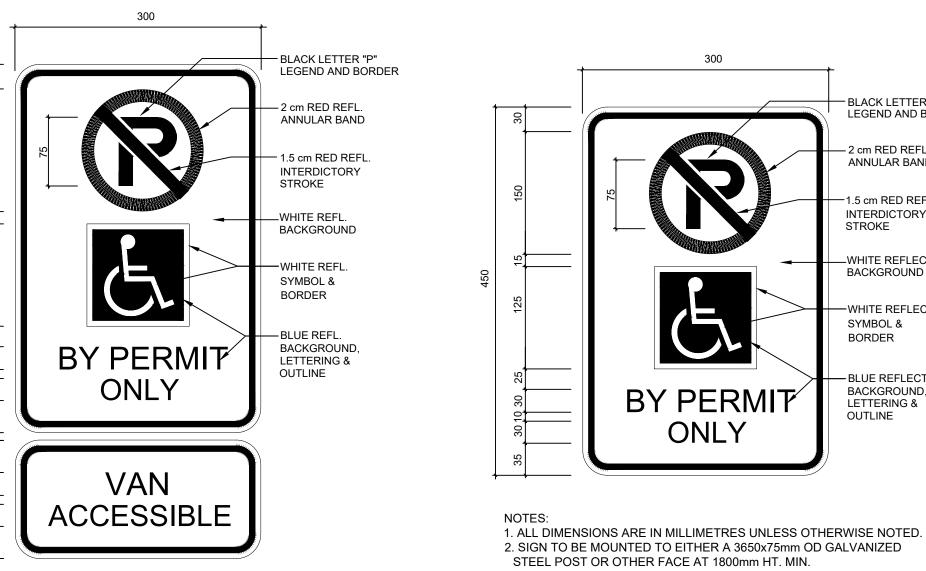
3. FONT HELVETICA BOLD CONDENSED. 1. ALL DIMENSIONS ARE IN MILLIMETRES UNLESS OTHERWISE NOTED. 2. SIGN TO BE MOUNTED TO EITHER A 3650x75mm OD GALVANIZED
