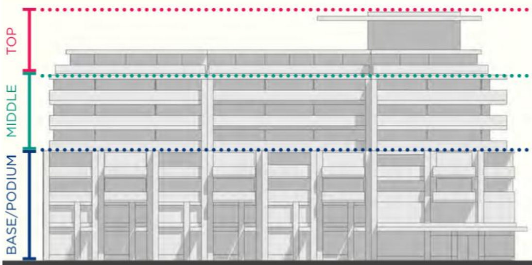
Figure 6 – City of Brampton Urban Design Guidelines – Components of a Mid-Rise Building (Source: City of Brampton / The Planning Partnership)
